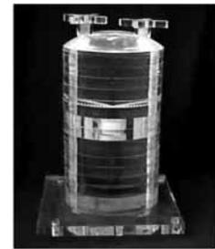
Figure 3. Plexiglass head phantom.
