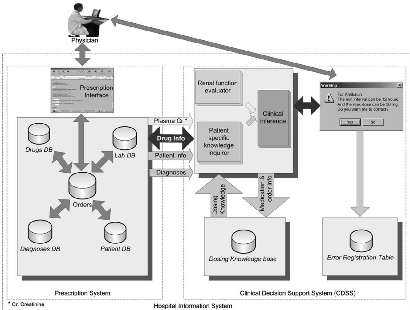
**Fig. 1** Schematic view of the CDSS architecture, and its interactions with the prescription system
